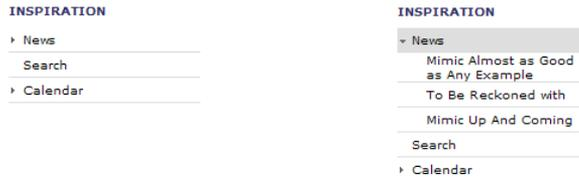
Figure 7-10: Menu created by Web Control Menu.ascx using Custom Controls PageTree and MenuList. The right-hand picture is the result of expanding the item News.
